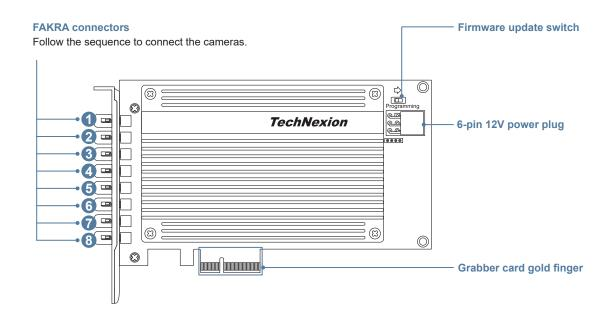
Note: To update the firmware, toggle the switch to the programming mode (right side) and strongly suggest operating this procedure by a technician.
