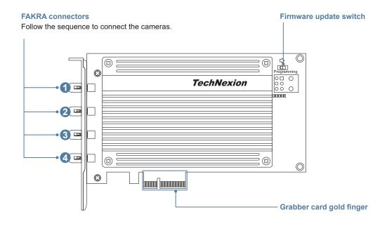
Note: To update the firmware, toggle the switch to the programming mode (right side) and strongly suggest operating this procedure by a technician.
