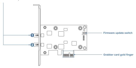
Note: To update the firmware, toggle the switch to the programming mode (right side) and strongly suggest operating this procedure by a technician.
