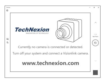
The camera isn't connected or detected. Please examine the connections between the camera, adapter, and computer.
