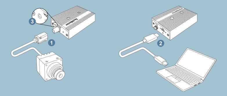
**Note:** Connect to a DC power adapter (10-30V/2A) with the size fit to 2.1x5.5mm plug if the computer you connected doesn't offer enough power to activate the adapter. Check the LED indicator status again once the extra power is connected.
